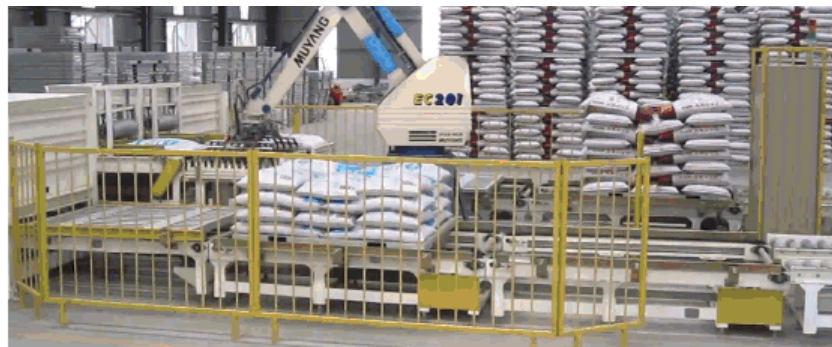
Robotic arms are used in Chinese feedmill warehouses.
